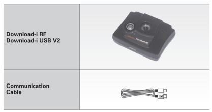
**Note:** The Download-i RF interface differentiates itself from the Download USB V2 because of the capability to read iButton and RFTags. This interface has an infrared reader.
